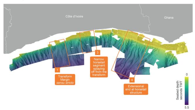
Figure 4 Seabed depth horizon (seconds, TWT) from PGS multi-client merged 3D seismic data highlighting three of the tectonic segment styles present offshore Côte d'Ivoire and Ghana as classified by Cronin et al. 2023. The approximate location of the three seismic lines in Figures 5-7 are indicated by the orange polygons 1, 3 and 4.
