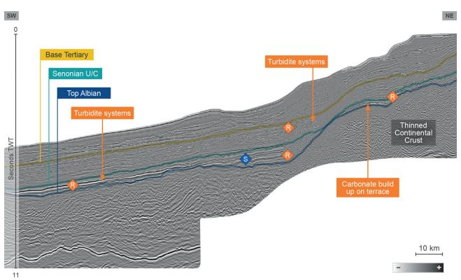
Figure 7 Merged 3D full-stack PSTM seismic dip line across tectonic segment 4: extensional end at horsetail segment (approx. line location indicated by polygon 4 on Figure 4). This line shows the extended lateral change from thin continental crust in the northeast to oceanic crust in the southwest with multiple ramp-terrace structures occurring along the shelf to deep water profile.
