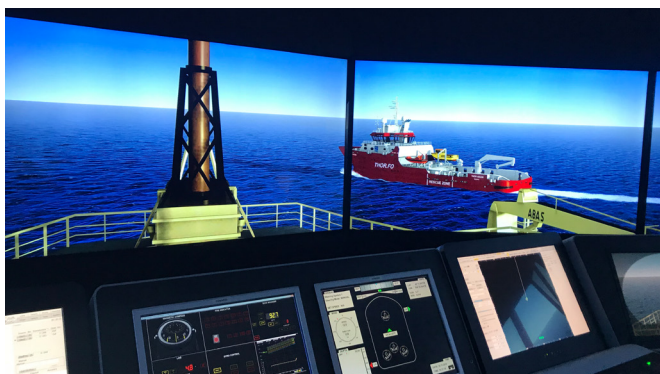
Figure 2. Simulation includes interaction between multiple vessels on the seismic operation. Here a support vessel passes the Ramform, and is manned by a team in a second bridge simulator.
