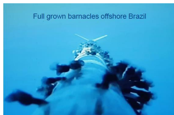
Figure 6: Underwater photo from the ROST showing advanced barnacle growth on a steamer with a three-wing steering and depth control device in the background.
