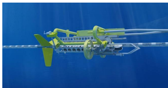
Figure 2: SCU passing a three-winged bird used for streamer depth and lateral control
