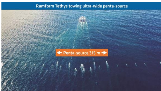
Figure 1. Overhead perspective of the penta-source configuration with 315 m outer source separation (above); and the ultra-near offset coverage over the 0-100 m offset class calculated from the navigation data belonging to two adjacent wide-tow source surveys in the Barents Sea in 2020 (right). The ultra-wide tow penta-source solution delivers almost gap-free live fold, while keeping the same efficiency. Refer also to the raw data comparison in Figure 2.
