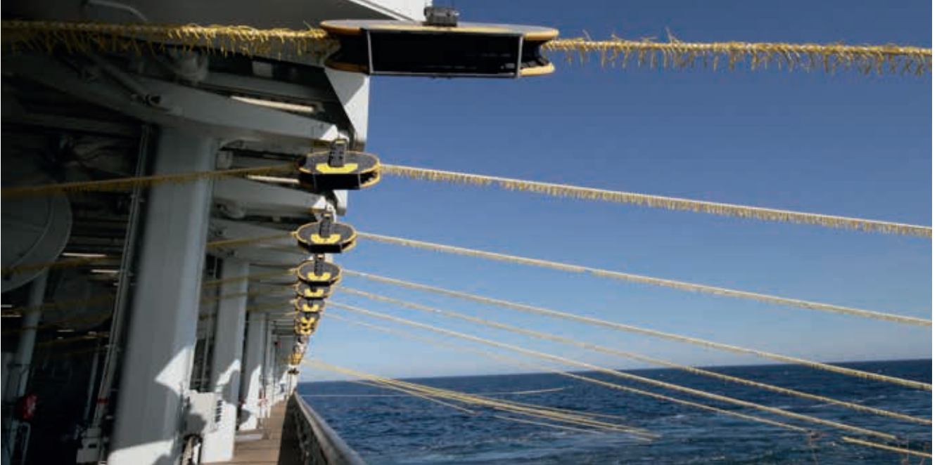
The Ramform Titan-class vessels have an aft stern of 70 meters. The vessels can tow 16 streamers with 100 meter separation and has 24 streamer reels onboard. The Ramform Titan-class vessels serves the ultra high-end segment of the seismic market.
