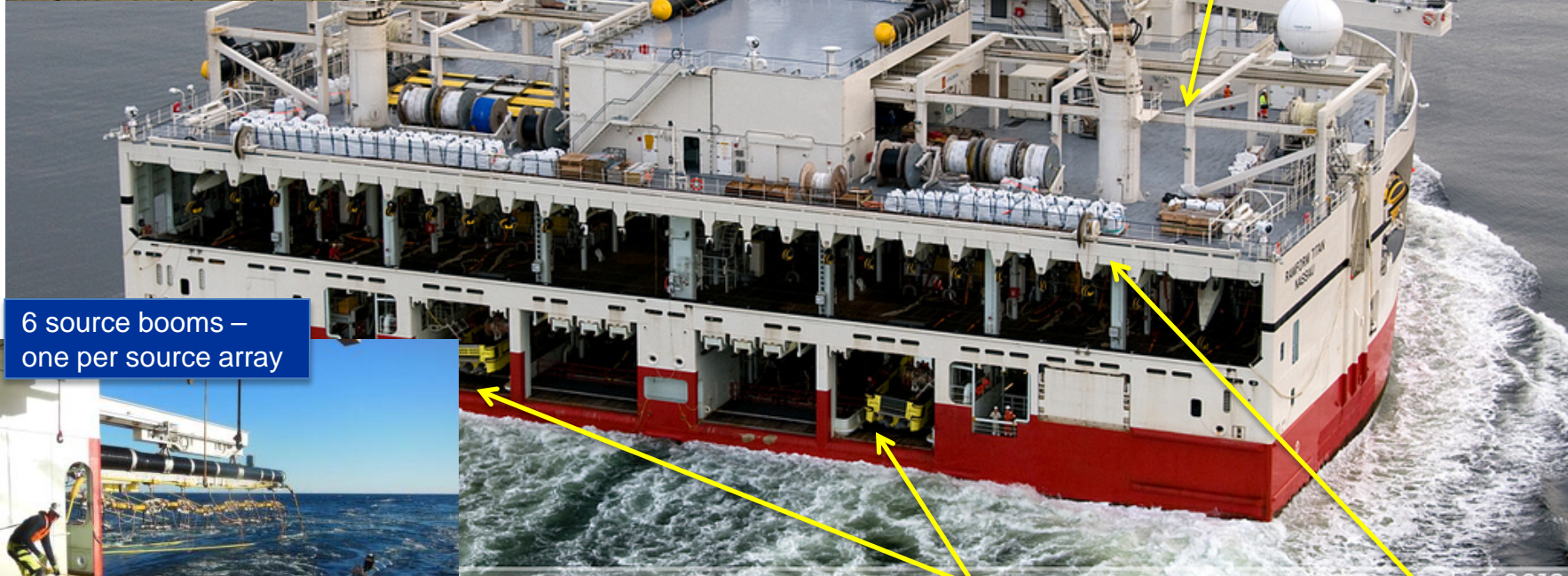
2 work boats in cradles deployed from stern of the vessel
