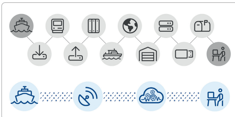
Figure 1 Traditional data flow (top) vs. optimised data flow (bottom). The traditional flow contains many data duplications and physical data handover points. The PGS optimised data flow transfers the subsurface information as soon as possible via satellite into the cloud for QC, processing and final delivery.
