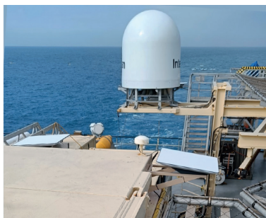
Figure 2 Left, LEO and GEO orbits relative to earth. Right, Starlink (front) and VSAT dome (back) satellite antenna on board the PGS vessel Vanguard.
