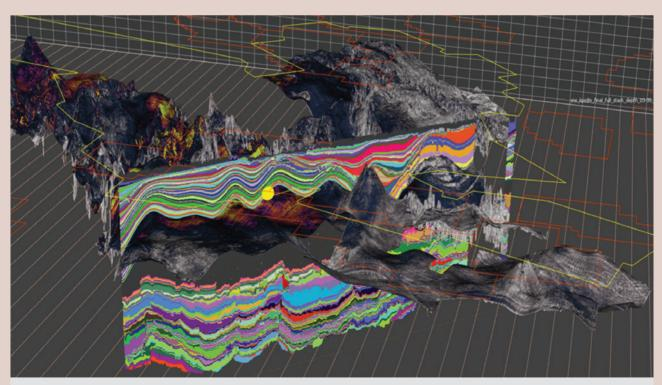
Figure 4. 3D representation of the Relative Geological Time model and the top of the salt over the 12 000 km² of reprocessed seismic data. The internal salt structure has been excluded from the seismic interpretation and the focus has been on the top and base salt. Interpretation RGT model produced using Eliis PaleoScan with PGS data.
